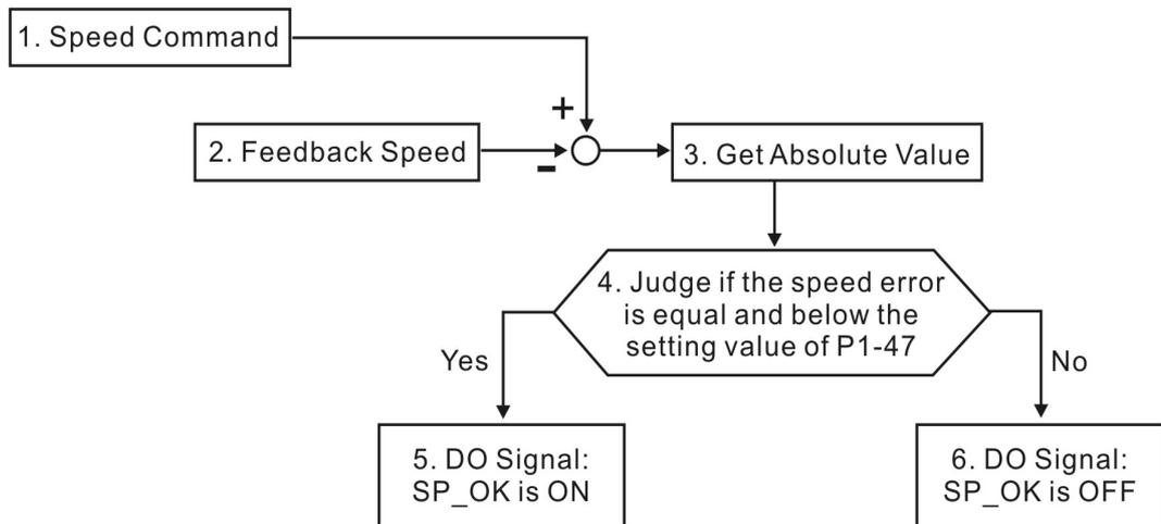
1. Speed Command: It is the speed command input by the users (no Accel/Decel), not the frond-end command of speed control loop. The source of this command includes analog voltage and registers.
