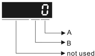
When the setting value of A is set to 0 or display is 0, it indicates that the load inertia estimation of semi-auto tuning mode has been executed but not been completed yet.
