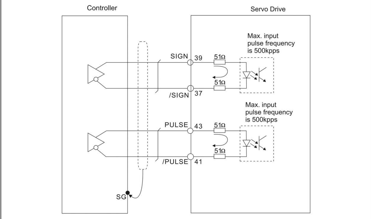
**C4-2: High-speed pulse input (Line driver).** It requires 5V power supply only. Never apply a 24V power supply.
