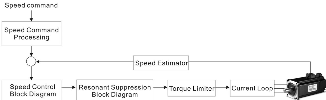
In the figure above, the speed command processing is used to select the command source of speed control according to chapter 6.3.1, including proportional gain (P1-40) and S-curve filter smoothing strategy of speed control. The speed control block diagram is used to manage the gain parameters of the servo drive and calculate the current input provided to motor instantaneously. The resonance suppression block diagram is used to suppress the resonance of mechanical system.
