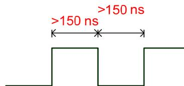
When the pulse frequencies of high-level duty and low-level duty both are greater than 150 ns, the signal will not be filtered (that is, the pulse command will pass through).
