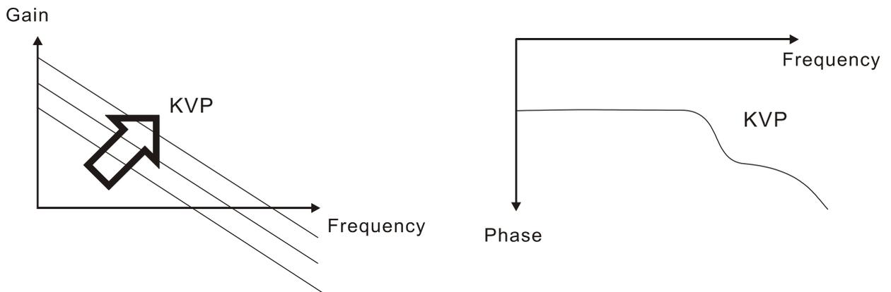
STEP 2 : Fix the value of KVP and adjust the value of KVI.
