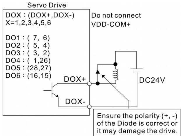
Use a relay or open-collector transistor to input signal.
