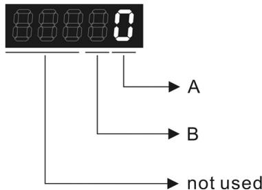
A: Analog monitor outputs polarity
