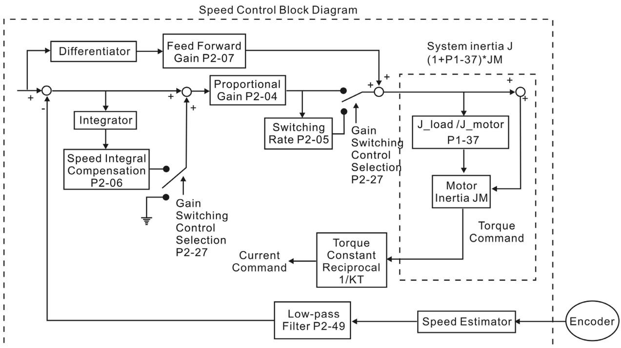
There are two turning modes of gain adjustment: Manual and Auto modes. The gain of ASDA-B2 series servo drives can be adjusted by using any one of three tuning modes.
