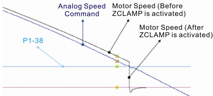
0: When the command source is an internal speed command, the users can use ZCLAMP DI signal to stop the motor at the desire position and keep the the acceleration and deceleration speed curve of the internal speed command. The motor will be locked at the position when ZCLAMP conditions are satisfied.
