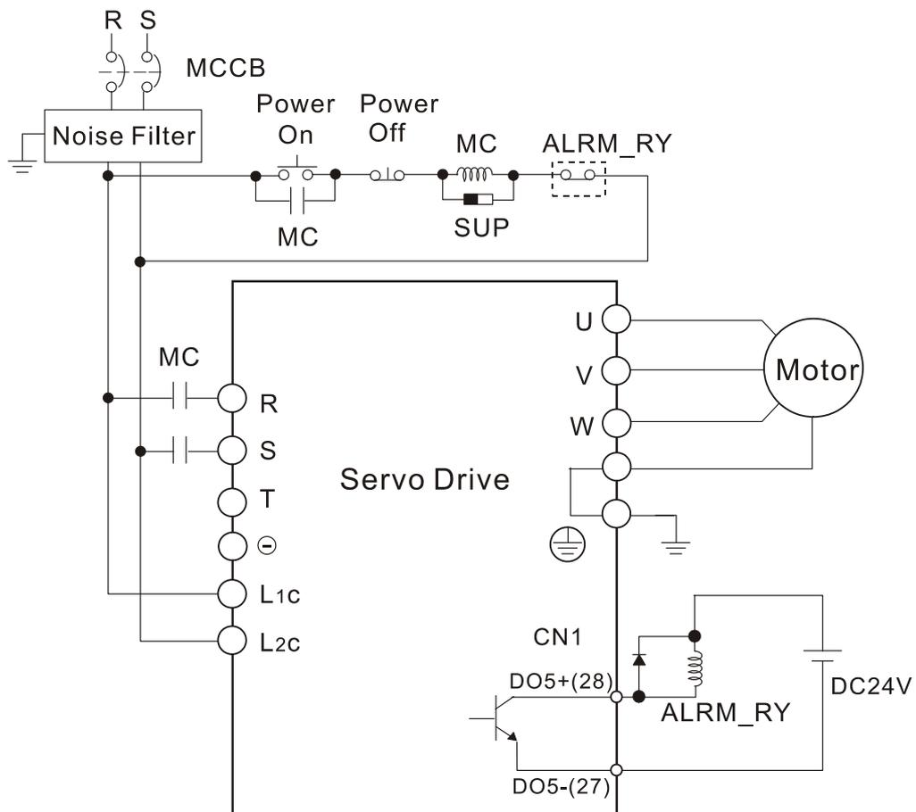
Figure 3.3 Three-Phase Power Supply (all models)
