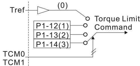
This parameter is used to determine that the speed and torque limit functions are enabled or disabled. If P1-02 is set to 11, it indicates that the speed and torque limit functions are enabled always. The users can also use DI signals, SPDLM and TRQLM to enable the speed and torque limit functions. Please note that DI signals, SPD0, SPD1, TCM0, and TCM1 are used to select the command source of the speed and torque limit.
