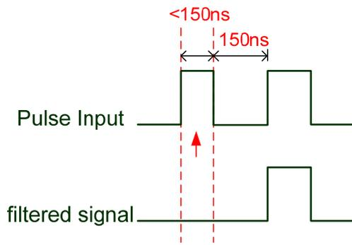
When this pulse frequency is less than 150 ns, this signal will be regarded as a low-level pulse and two input pulses will be regarded as one input pulse.
