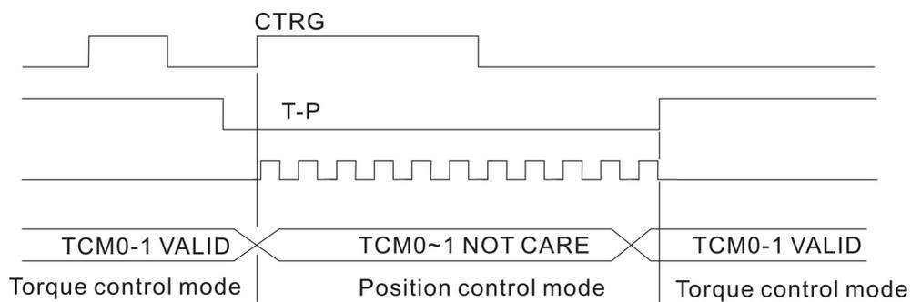
Figure 3. : Torque / Position Control Mode Selection
