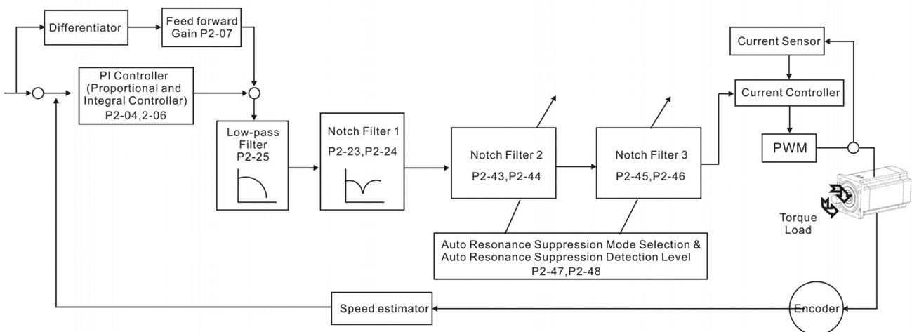
There are two groups of notch filters provided by ASDA-A2 series. The first group of notch filter is P2-43 and P2-44, and the second group of notch filter is P2-45 and P2-46. When there is resonance, please set P2-47 to 1 or 2 (Auto mode), and then the servo drive will find resonance frequency and suppress the resonance automatically. After suppressing the
