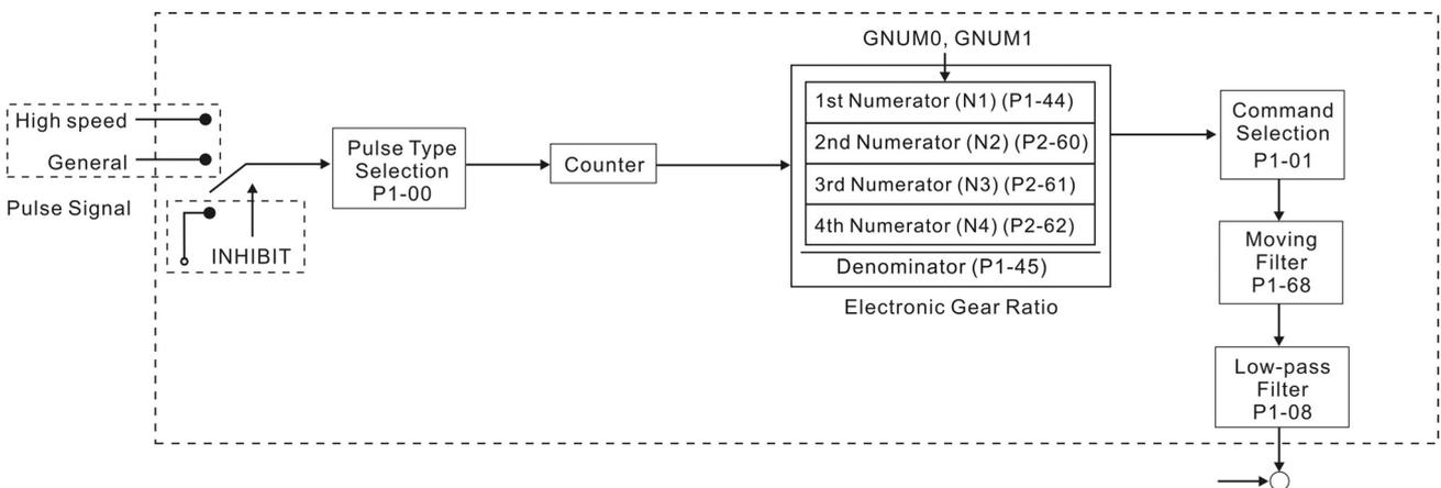
Using parameter P1-01 can select P mode. Electronic gear ratio can be set in P modes to set proper position revolution. ASDA-B2 series servo drive also provides low-pass filter, which are used whenever the motor and load need to be operated more smoothly. As for the information of electronic gear ratio, and low-pass filter, please refer to the following sections 6.2.3 and 6.2.4.
