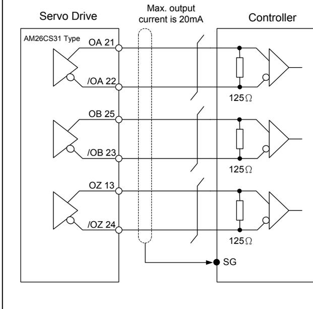
**C14: Encoder output signal (Photocoupler)**
