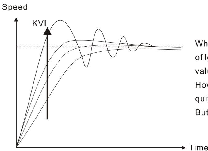
When the value of KVI is greater, the value of low-frequency gain is also greater and the value of steady error is nearly zero (0). However, the value of phase margin will reduce quite substantially. It is helpful to steady error. But it is not helpful to dynamic tracking error.
