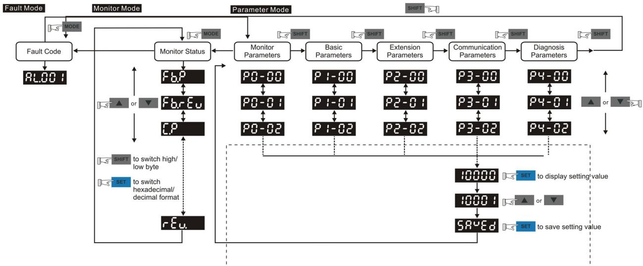
1. When the power is applied to the AC servo drive, the LCD display will show the monitor function codes for approximately one second, then enter into the monitor mode.
