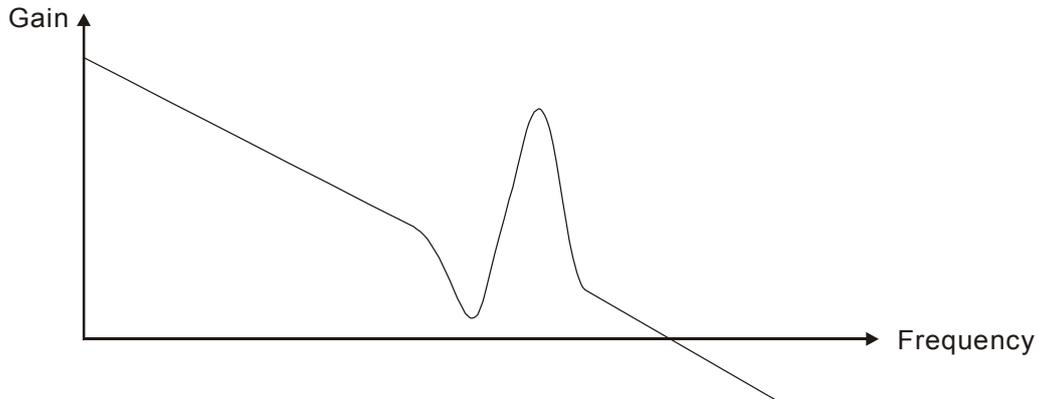
When the low-pass filter (parameter P2-25) is adjusted from 0 to high value, the value of Low-pass frequency (BW) will become smaller (see the figure below). The resonant condition is improved and the frequency response and phase margin will also decrease.
